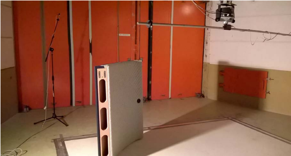
Figure 1. Single panel with phonix in place for testing
